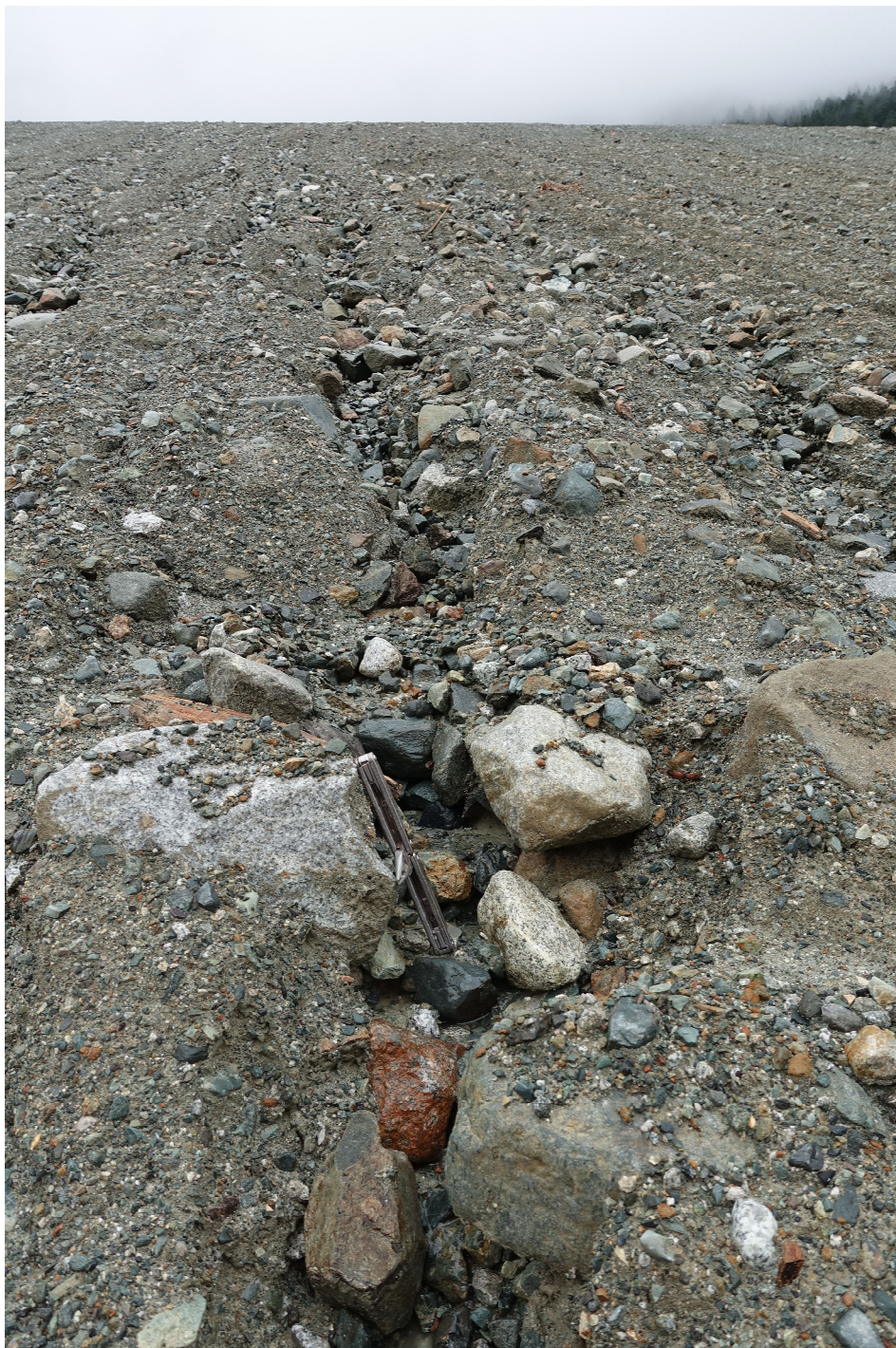
Figure 5. Erosion rill on the Lynx TDF closure cover trial (multi-tool for scale—tool is 20 cm from one end of the handle to the other).
