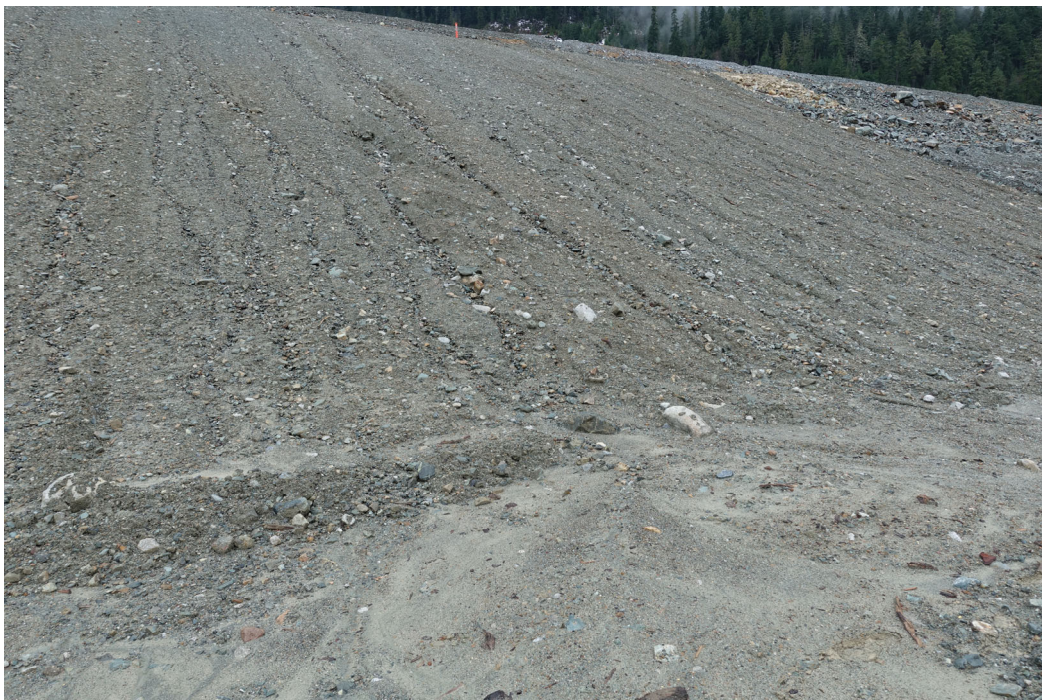
Figure 4. Erosion rills and deposition fans on the Lynx TDF closure cover trial.
