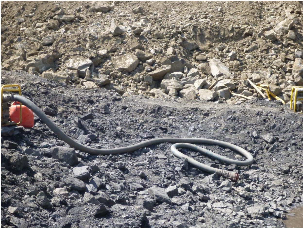
Figure 4 – Hose used to pump out fuel. It is also full of fuel that needs to be disposed of.
