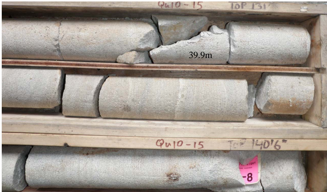
Photo 7: DH QU10-15, 39.9m depth. Pre-existing fracture 20 degrees TCA with fe stain.
