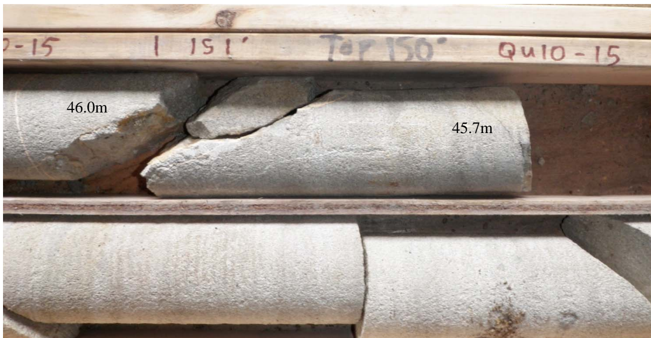
Photo 10: DH QU10-15. 45.7m depth open micro-fracture 65 degrees TCA. 46.0m depth fault with trace gouge, fe stain, calcite coating
