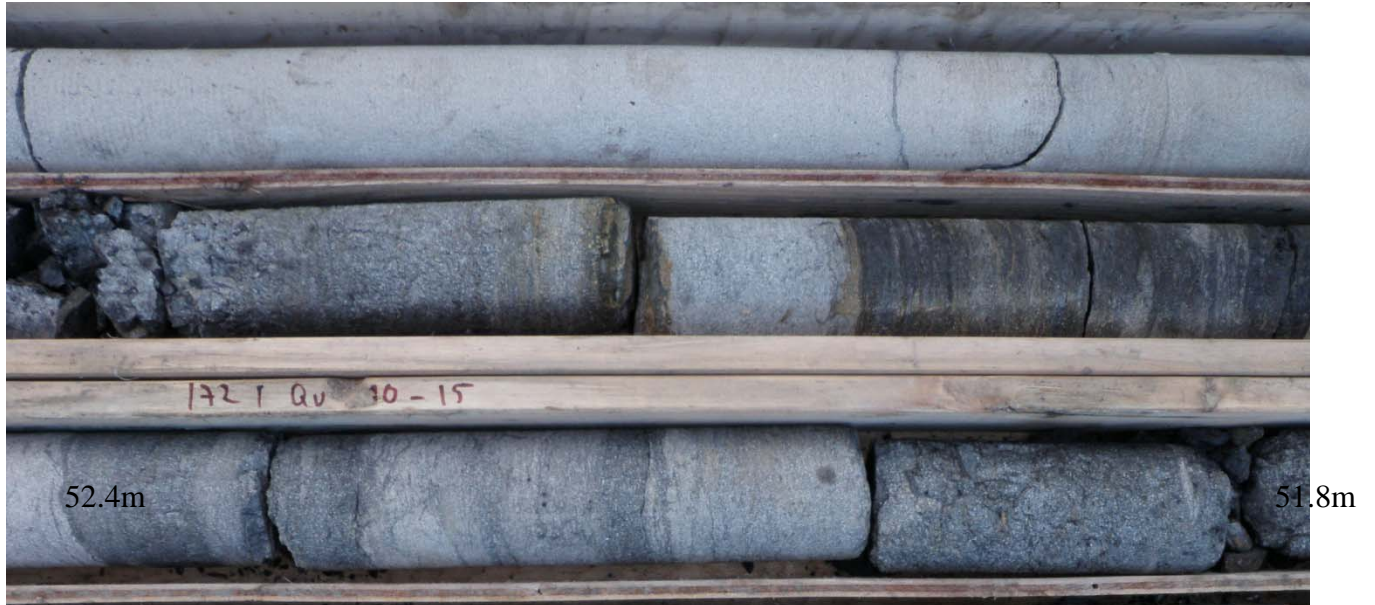
Photo 11: DH QU10-15 51.8m to 52.4m open micro-fractures in carbonaceous sandstone
