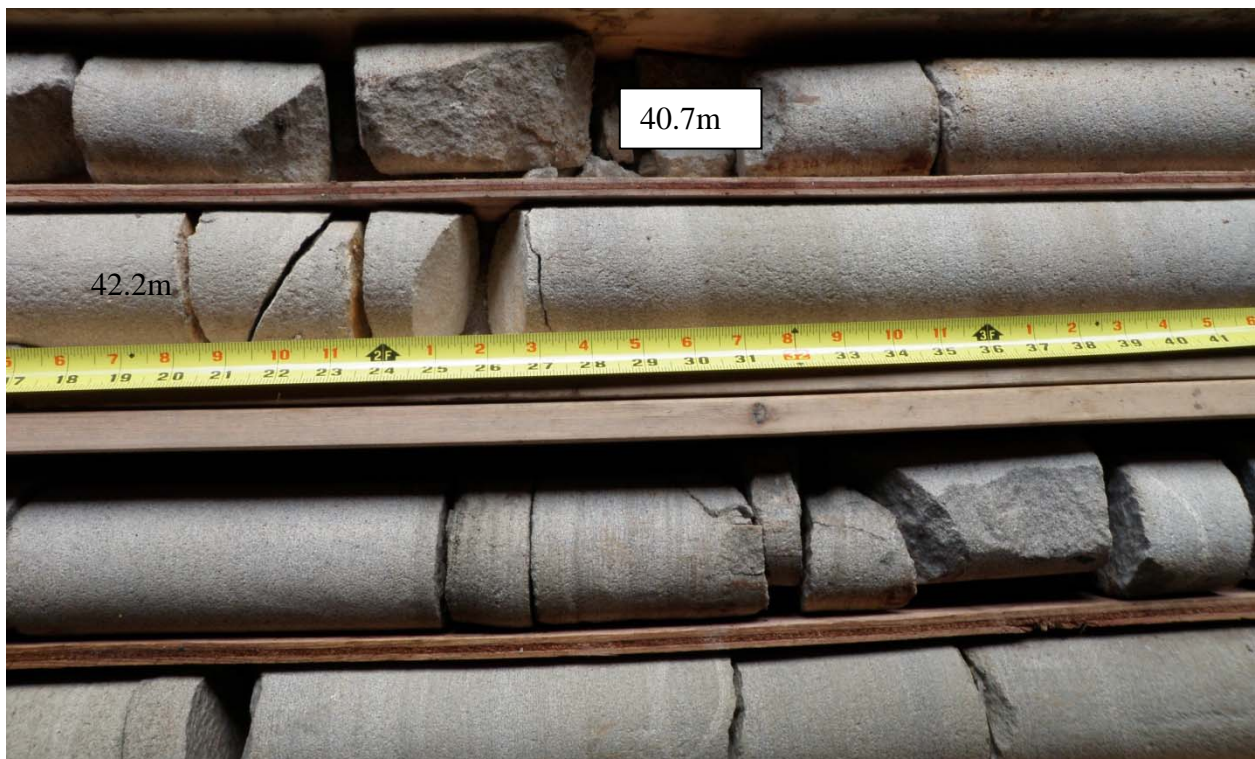
Photo 8: DH QU10-15. 40.7m depth, joint/fault 15 degrees TCA with trace gouge (non softening). 42.2 joints at 85 and 65 TCA with Fe stain
