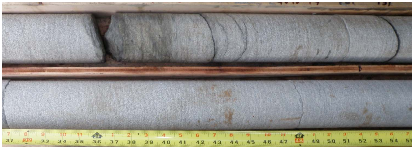
Photo 12: DH Qu10-17 46.5m. Open micro-fractures on dark mineral bands
