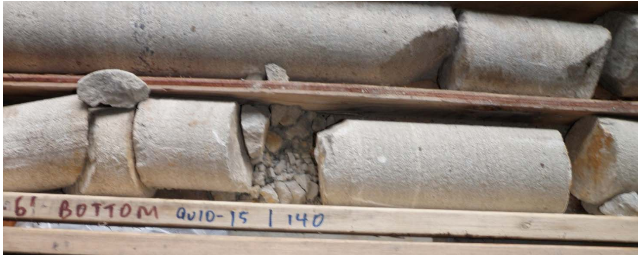
Photo 9: DH QU10-15. 42.7m (140 ft) depth . 30mm fault zone with gouge and rubble on bedding plane
