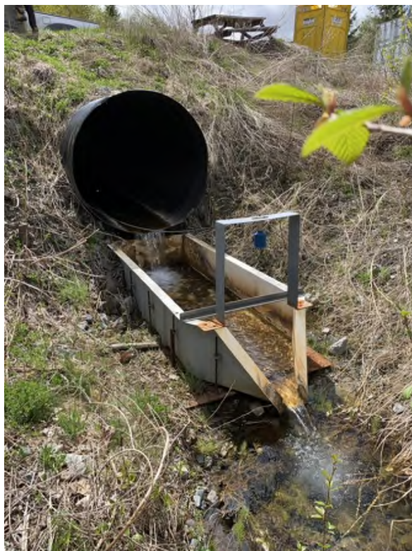
Photo 21: 3 South Pit Inlet Flow Measuring Weir, Immediately Downstream of Access Road.
