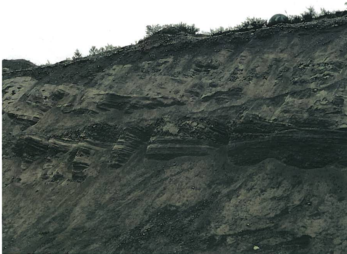
Figure 6: South pit wall, distinct near horizontal layering observed, vertical hydraulic conductivity may be significantly less than horizontal hydraulic conductivity
