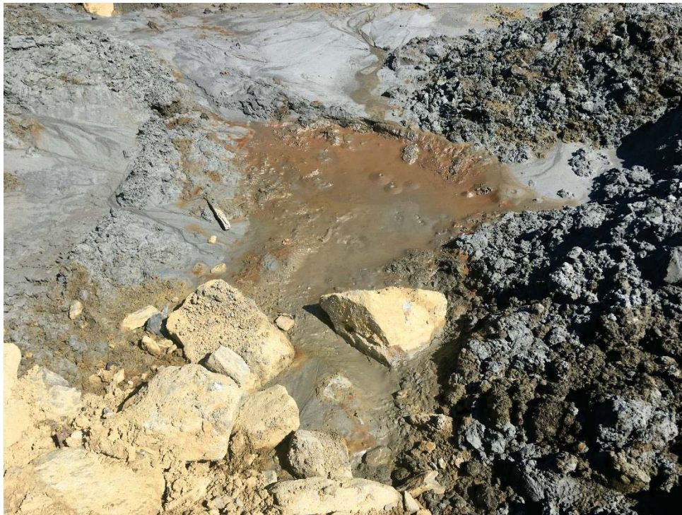
Photo 8: Indications of upwelling groundwater at the upstream toe of Lynx TDF construction, in response to consolidation (22 July)
