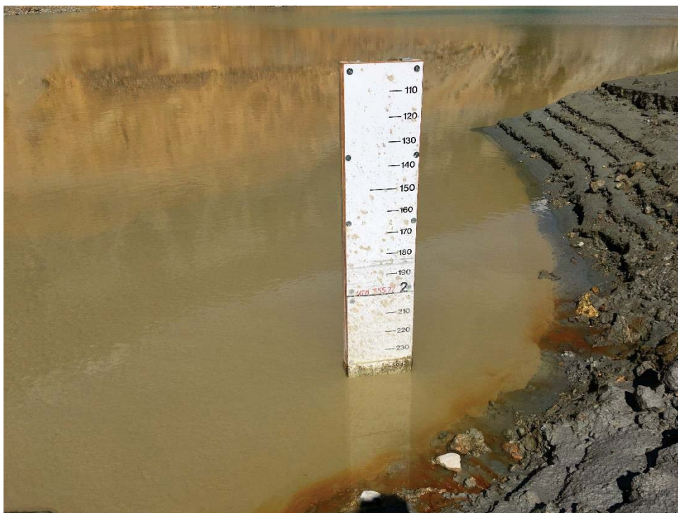
Photo 5: Staff gauge in Lynx TDF. Clear water level is 2.40 on the gauge. Sediment laden water level is 2.44 on the gauge. (29 July)
