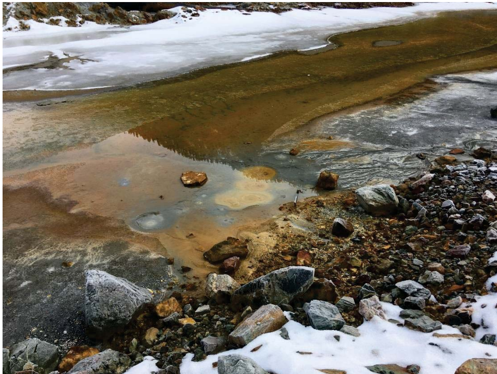
Photo 2: Groundwater boils in the East Strip. Light to moderate activity.
