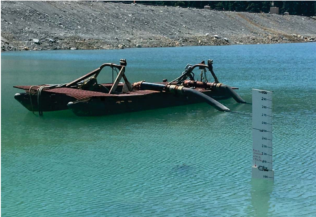
Photo 5: Water level in Lynx TDF is 1.88 on the staff gauge, 356.19 m elevation. Maximum Normal Operating Water Level is 355.0 m.
