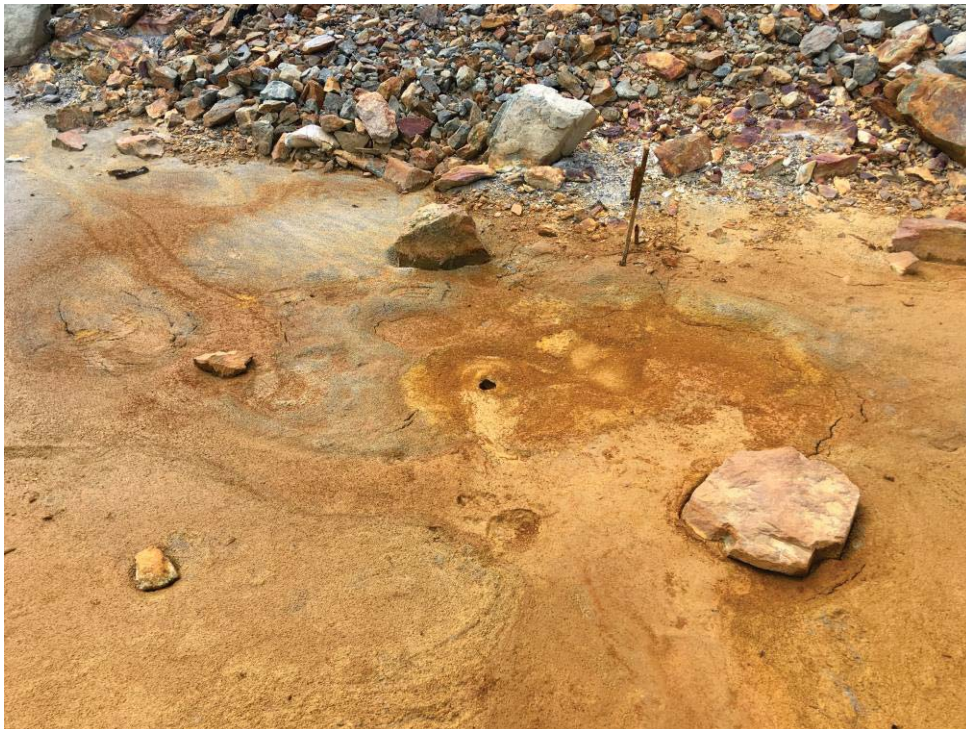
Photo 2: East Strip boils are dry. Some indication that flow may have reversed, with these springs acting as sinks.
