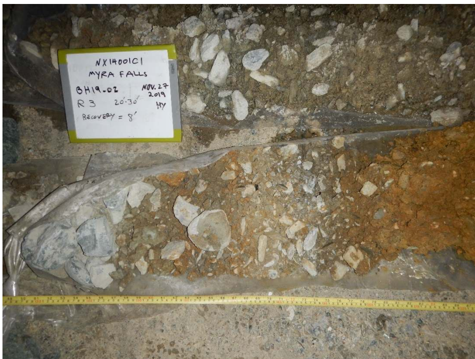
PHOTO 24: BH19_02 Representative Sample Depth 20'-30' (November 27, 2019)
