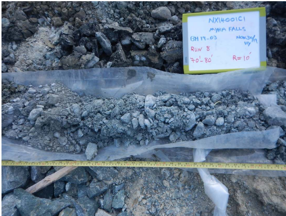
PHOTO 43: BH19_03 Representative Sample Depth 70' - 80' (November 30, 2019)
