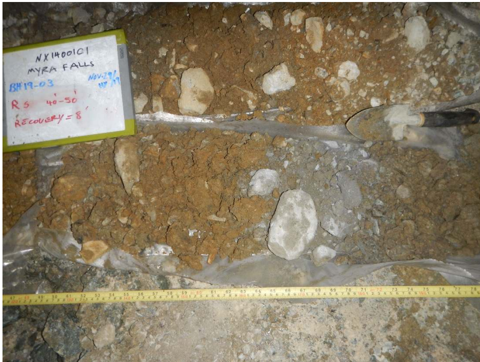
PHOTO 39: BH19_02 Representative Sample Depth 40' - 50' (November 29, 2019)
