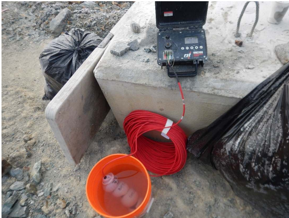
PHOTO 51: BH19_03 VWP Initial readings prior to Installation (December 1, 2019)
