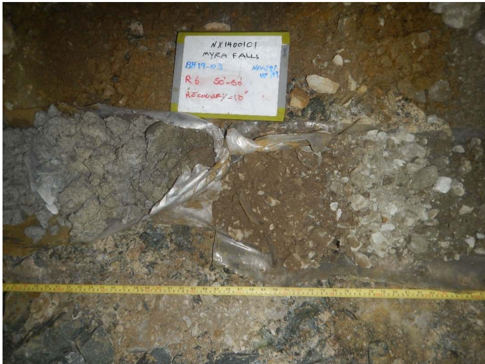
PHOTO 40: BH19_02 Representative Sample Depth 50' - 60' (November 29, 2019)
