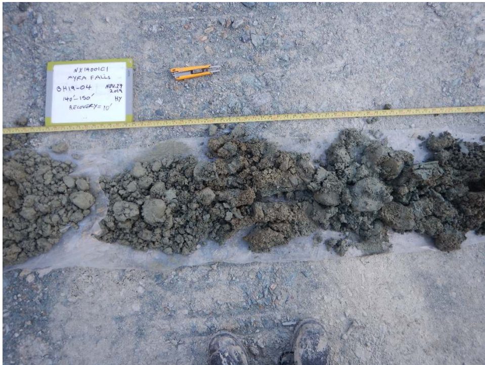
PHOTO 21: BH19_04 Representative Sample Depth 140'-150' (November 27, 2019)
