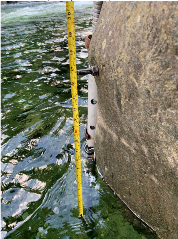
Plate 3. MYR-BDG-US, recording stage using a surveyed reference mark (January 27th, 2020)
