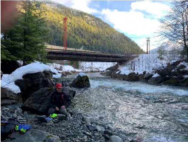
Plate 1. MYR-BDG-US during a salt dilution discharge measurement (January 27th, 2020)
