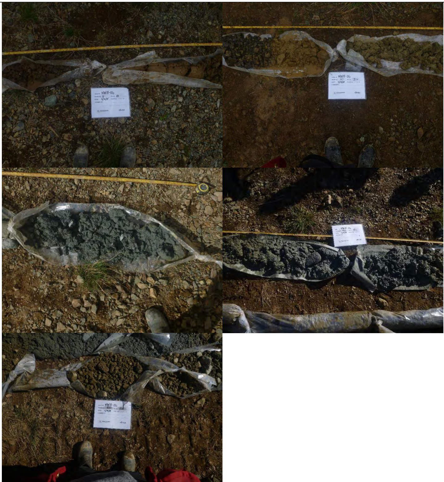
Photo 5: Soil cores at MW18-06S/D (from 0' to 60').
