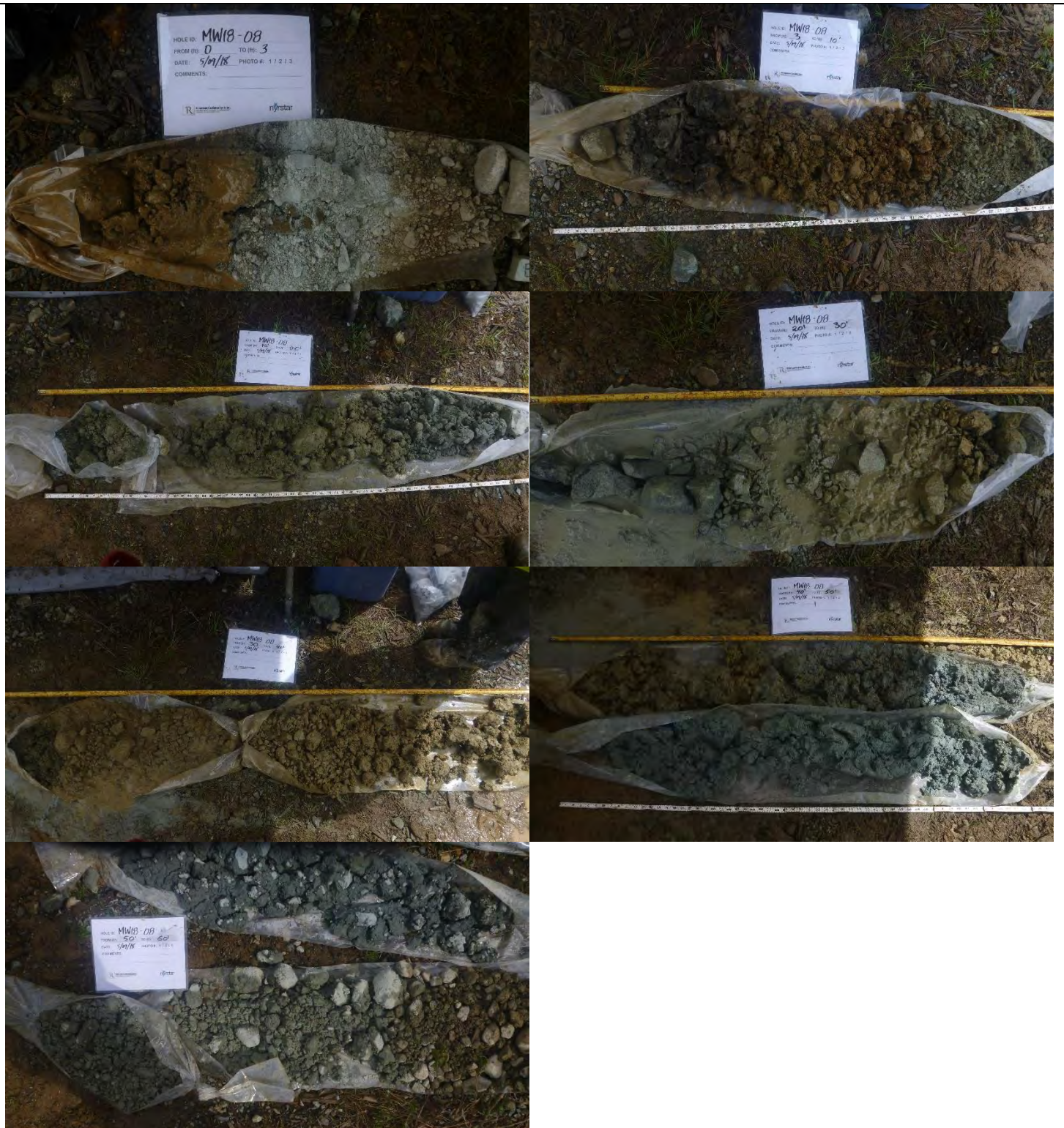
Photo 7: Soil cores at MW18-08S/D (from 0 to 60').
