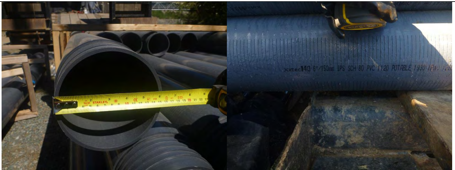
Photo 3: 6" Schedule 80 PVC (left) and 20-slot screen section used for pumping well installations (right).
