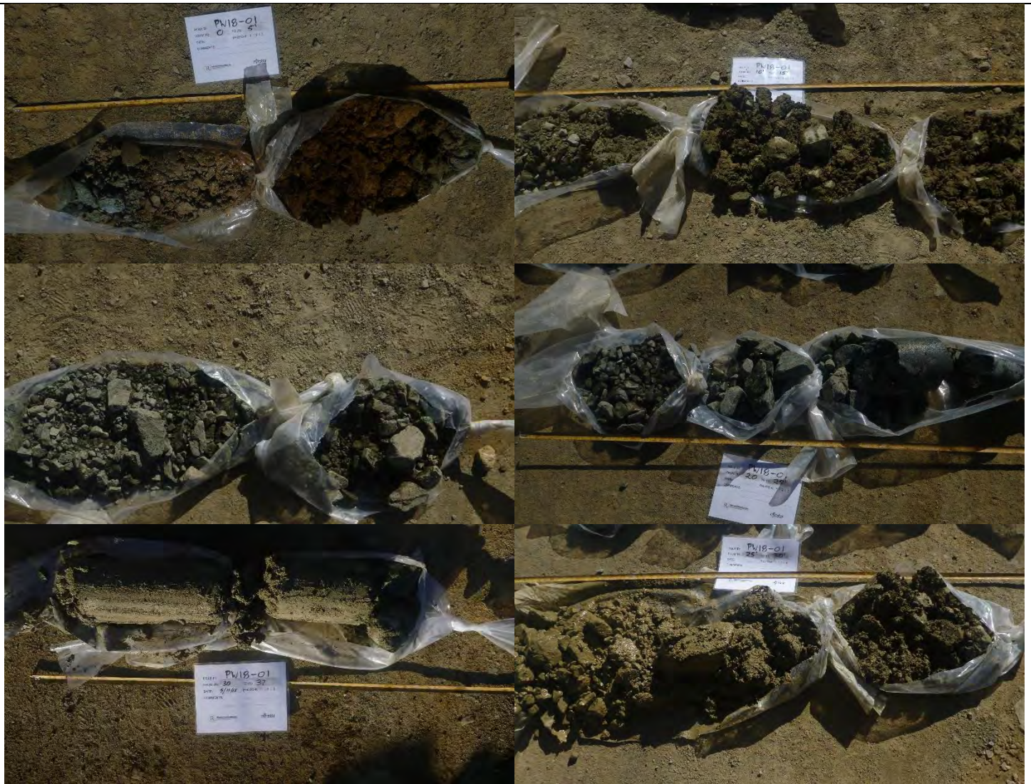
Photo 8: Soil cores at PW18-01 (from 0 to 37').
