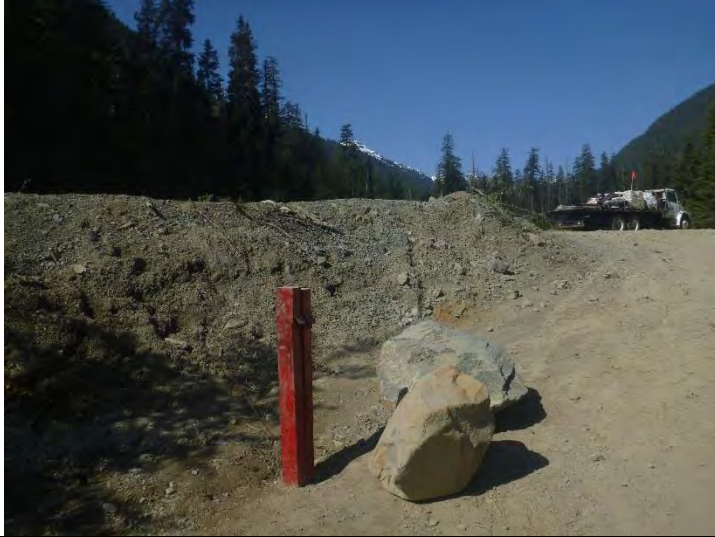
Photo 6: 2" monitoring wells with red protective casing at MW18-06S/D (top left), MW18-07S/D (top right), and MW18-08S/D (bottom left). All locations are nested installations with both shallow and deep wells installed together in one borehole.
