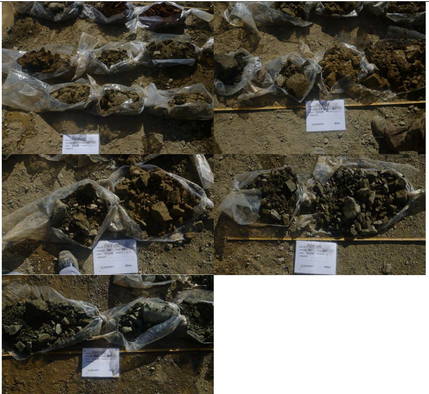
Photo 10: Soil cores at PW18-03 (from 0 to 37').
