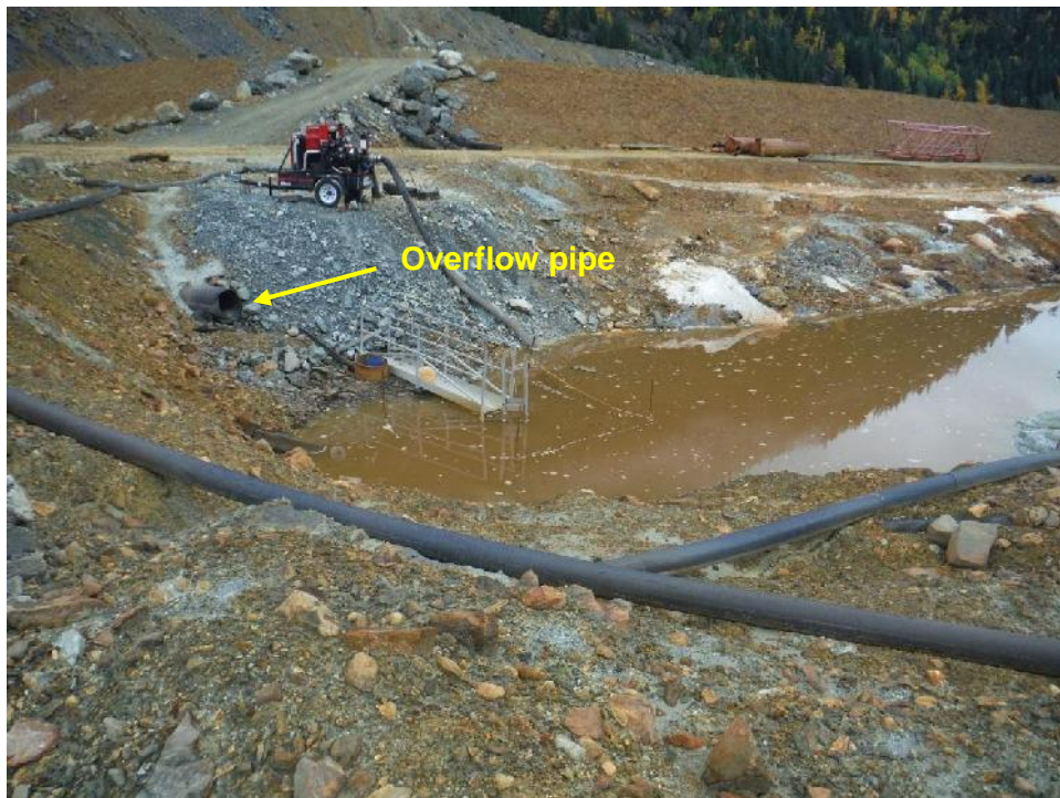
Photo 16 – West Strip decant structure and overflow pipe with four inch pump.
