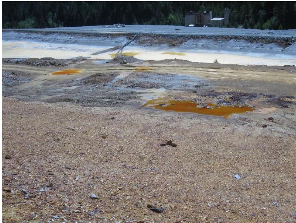
Photo 7 – ARD seepage at the toe of the Paste Berm near Instrument Plane 4, looking south. East Strip in the background.
