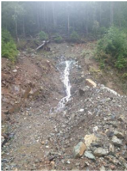
Photo 39 – Significant flow over the bedrock at the Arnica – Upper Lynx Diversion junction, infiltrating into ground and continuing into Lynx pit.
