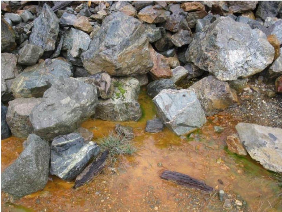
Photo 25 – Close-up view on a seepage location source on the mid-level bench of Lynx Dam south arm.
